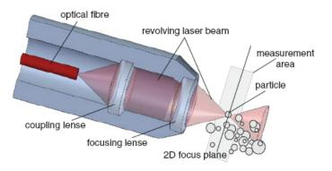
**Figure 8.** (a) Design of the fiber optical FBR sensor: 3D drawing of the tip of the probe (*left*) and the cross-section of the probe (*right*); (b) A FBRM probe using light back scattering effects for drop sizing [99].
