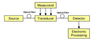
Figure 1. Basic components of a fiber-optical sensor system [25].
