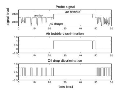
Figure 4. Probe detection and data processing for air bubbles in oil-in-water flow [43].
