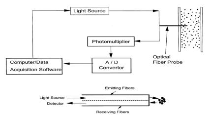
Figure 6. The fiber-optical probe system for solids holdup measurement.
