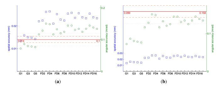
We only reach the simulation results for the angular accuracy when the Gom is in the target frame. The spatial accuracy is also much better for these five positions, rarely exceeding 10% more than the
