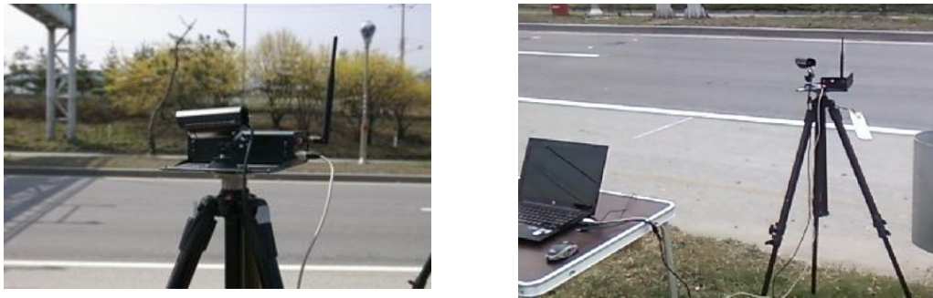
(e) T-BS-com node with a video camera and the T-Mon Host
