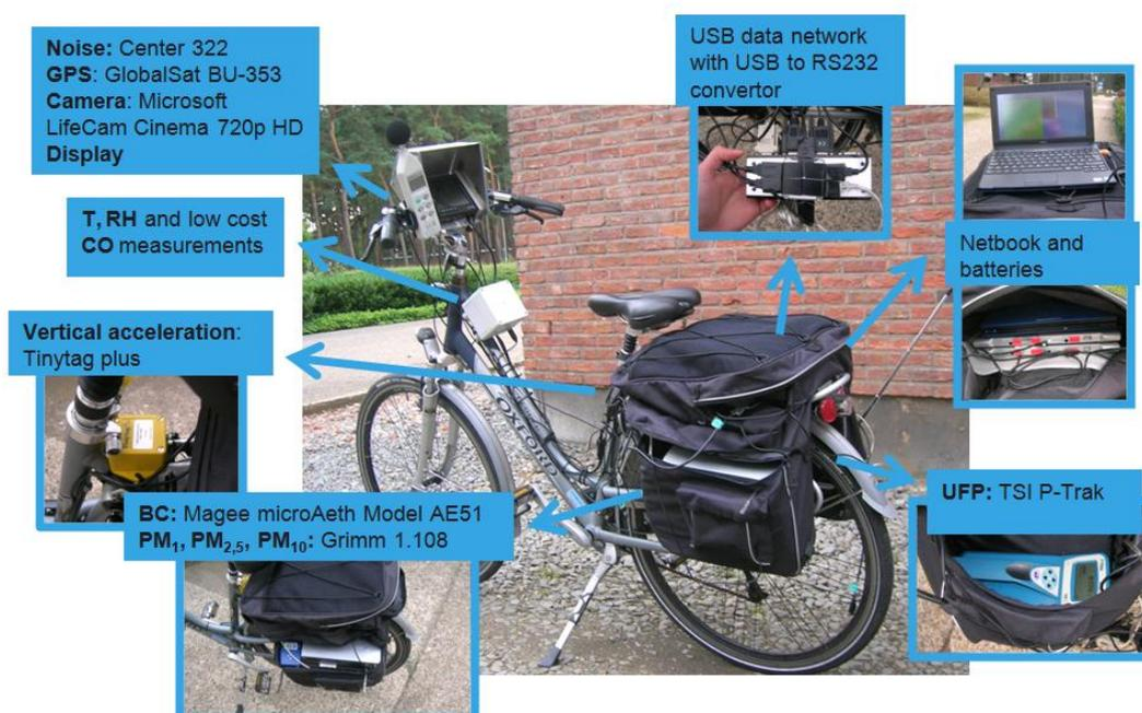
All selected air quality measurement devices are able to transmit their measurements in real time to a computer. Also, their power usage requirements are low enough to power them by batteries. Springs and foam are used to protect the sensitive optical measurement devices from shocks during the measurement ride. Furthermore, the Aeroflex is equipped with a number of additional measurement devices: a GlobalSet BU-353 GPS with SiRFstarIII chipset, a Center 322 sound level meter, a
