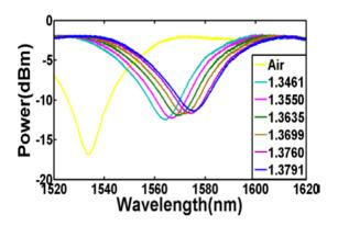
**Figure 5.** Wavelength response for different external refractive index ( $D = 60 \mu m$ ).
