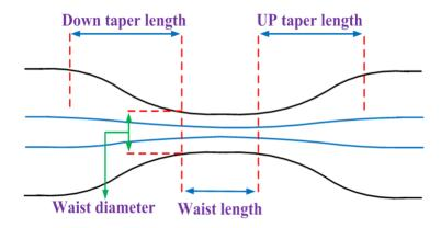
Figure 1. Schematic view of taper profile.
