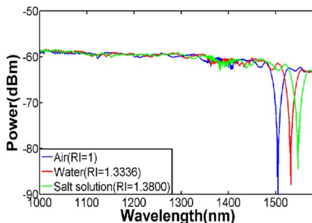
**Figure 7.** RI sensitivity characterization for both sensors ( $D = 60 \mu\text{m}$  and  $D = 55 \mu\text{m}$ ).
