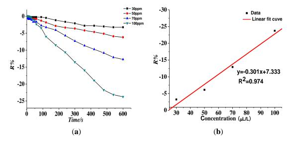
(3) Response of the gas-sensing characteristics of the Pt-doped TiO<sub>2</sub>NTs gas sensor to  $SF_6$  partial discharge decomposition component  $SO_2F_2$ .
