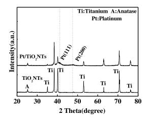
Figure 5. XRD of the Pt-doped TiO<sub>2</sub>NTs.
