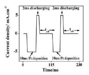
Figure 1. Current-time curve for the preparation of Pt-doped TiO<sub>2</sub>NTs.
