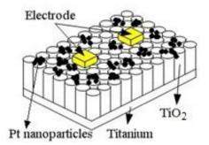
2.3. Gas Sensing Test Device and Method for the TiO<sub>2</sub>NTs Sensor
