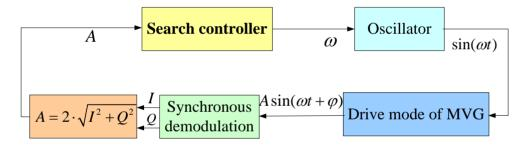
Figure 4. The principle diagram of the synchronous demodulation technique.
