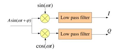
• The synchronous demodulation module is adopted to obtain the amplitude of the response signal, whose principle diagram is presented in Figure 4. Obviously:
