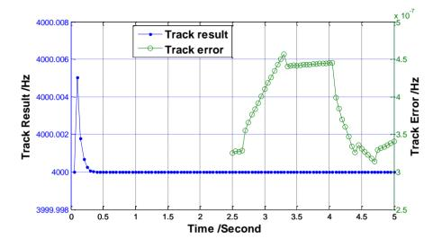
The second simulation is carried out to evaluate the performance for tracking varying frequency, where the resonant frequency changes linearly with a 10 Hz/s slope from 4,000 Hz to 4,050 Hz. The results are plotted in Figure 11, which shows the relative error is about 5e-5.
