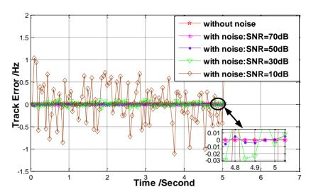
Figure 12. Errors of the track method under different level noise ( $f_r = 4,000$  Hz).
