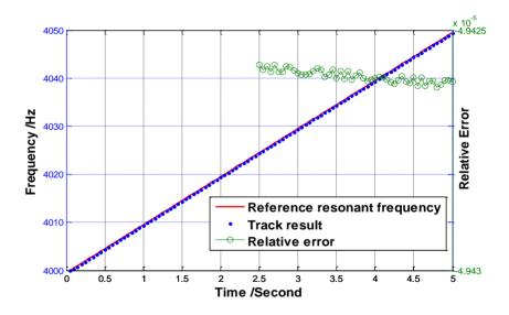
Finally, the performance of noise resistivity is simulated. The resonant frequency here is still set as a constant ( $f_r = 4,000$  Hz), and random noise determined by the SNR is added to the detected phase. Track errors under different level noise are presented in Figure 12. It is obvious that the track method behaves well but its measurement precision decreases. When SNR = 50 dB, the measurement error is less than 0.01 Hz.
