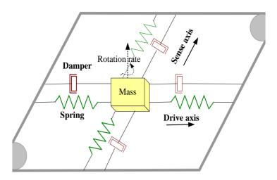
In the drive direction, a controlled sinusoidal force is generated to make the mass vibrate at the drive-mode resonant frequency and achieve stable amplitude by the use of the automatic gain control (AGC) method [17]. When an angular rotation around the input axis exists, a Coriolis force will be formed. The force causes a vibration in the sense direction. Ideally, the dynamics of MVG can be described as follows [16]:
