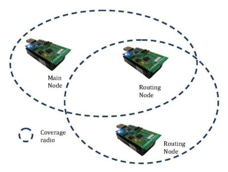
We propose implementing a network as presented in Figure 11, which consists of 3 fixed nodes that will not have power consumption restrictions. These three nodes will receive the reports transmitted by the sensors located on five patients that route the message to the sink node. Fixed nodes have identifiers 0, 1 and 2 and the sink node has the ID 0. Patient devices have IDs from 3 to 7.
