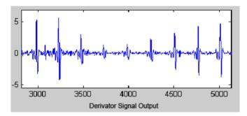
Previously, to carry out the window integration process, the quadratic function was applied for all signal points to be converted into positive values that emphasize the high frequency signal, which is mainly the QRS complex (Figure 6).
