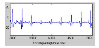
After the signal is filtered, most of its energy is contained in the QRS complex. Then, the derivative function is applied, high frequencies are accentuated and the low frequencies are attenuated. Therefore, the high slopes are highlighted to generally distinguish the QRS complex within the ECG signal.
