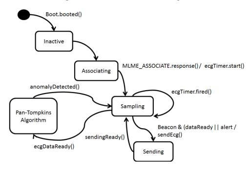
Figure 13. Network Device State Diagram.
