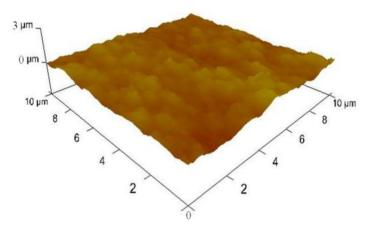
It shows a dramatic contrast from the surface roughness of plain platinum surface right after e-beam evaporation which was found to be  $0.493 \pm 0.3$  nm. This result shows that the platinum nanoparticles electrodeposited on collapsed entangled MWCNT forest greatly increased the surface roughness. In
