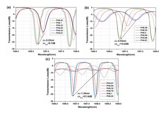
Figure 6 gives the spectral evolution of our fiber-optic sensors with pH for different thicknesses of sensing film. For each film, the pH of the aqueous solutions was adjusted by HCl or NaOH solution (in the range from 3.4 to 7.24). It can be seen that the pH increases, the coupling strength of the cladding mode resonances also increases. The reason is that with increasing pH, more carboxyl groups
