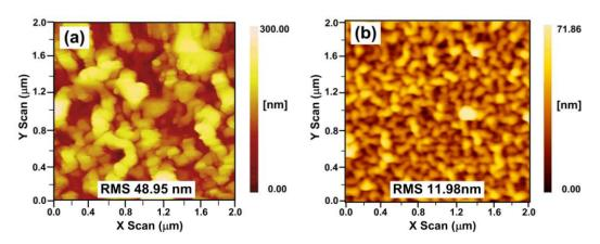
Figure 2 gives the atomic force microscopy (AFM) images of (PDDA/PAA)<sub>4</sub> and (PDDA/PAA)<sub>10</sub> multilayer films (dry). A wormlike or vermiculate pattern can be observed for the multilayer, which is a general phenomenon for common polyelectrolyte multilayer films [3,18]. However, comparing Figure 2(a,b), the morphology of the (PDDA/PAA)<sub>4</sub> multilayer film has smaller, less connected
