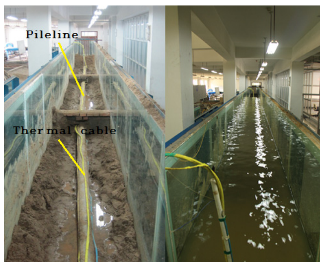
Figure 7. Experimental set-up: the thermal cables were placed in the vicinity of the pipeline ( left ) and the system operated in running water environment ( right ).
