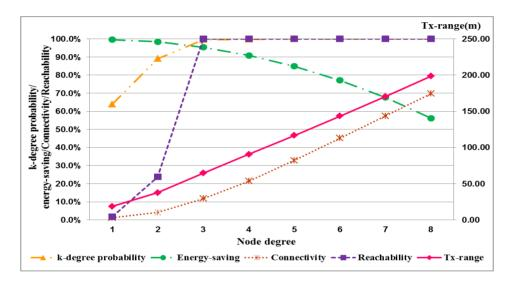
**Figure 5.** The corresponding relationship of network evaluations with a node density of  $0.005 \text{ nodes/m}^2$ .
