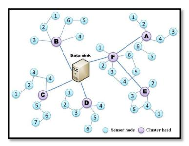
A component is a node set, in which there is at least a path between two arbitrary nodes. In a component, all nodes can deliver data each other. In a network with only a component, the network topology is full reachability. If the network topology is formed by many components, the network reachability is decreased. Hence, the transmission range is the key point for component number in a network. And the network topologies also are produced through the transmission range. To evaluate
