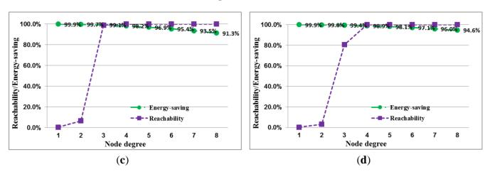
**Figure 9.** A comparison of simulation results for the transmission range with node degrees ranging from 1 to 8 with different node densities.
