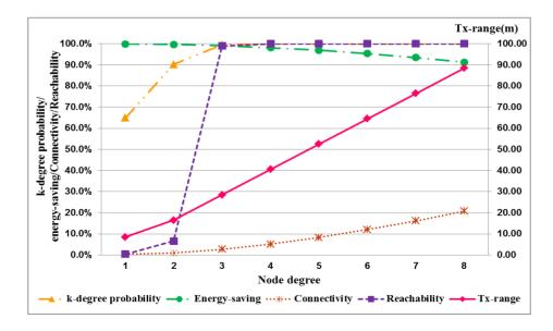
The performance index curves for the connection quality of a network with different node densities are shown in Figure 6. The two curves imply the relationship of reachability and connectivity of network.
