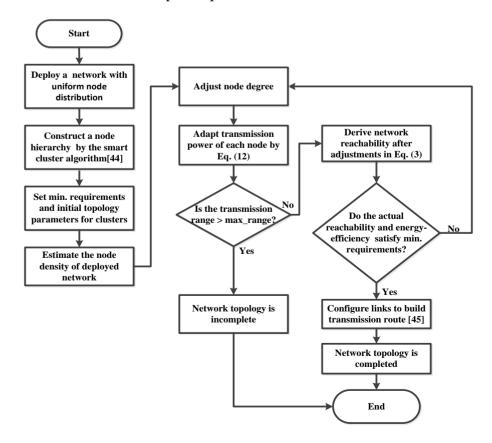
In cooperation with the authors' previous work of the smart cluster algorithm [44] and the routing algorithm [45], a high energy efficiency WSN is obtained through the steps as follows.
