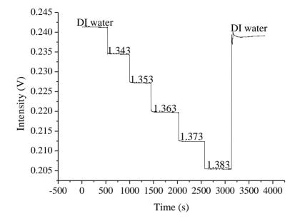
Figure 24. Plot of the PPR fiber sensor response *versus* the refractive index of the sucrose solution.
