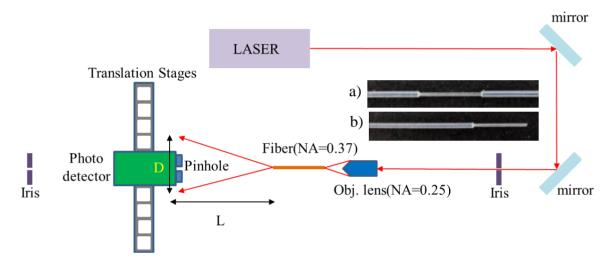
Figure 12. Schematic of the numerical aperture measurement instrument.
