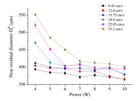
To ensure a residual diameter of nearly  $400 \ \mu m$  using laser processing while avoiding the non-processed removal of material from the fiber core layer, we established an acceptable range for the residual diameter:
