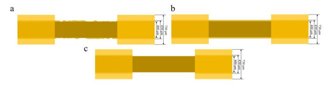
Figure 6. Schematic of optical fiber defects: (a) non-uniform changes in property; and (b) uniform changes in property.
