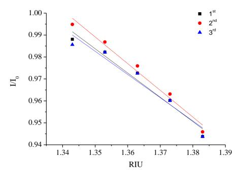
Figure 22. Plot of the ATR fiber sensor response *versus* the refractive index of the sucrose solution.
