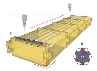
The yellow portion of the structure shown in Figure 3 is the optical fiber to be processed, the blue dotted line denotes the established processing direction of the optical fiber, and the red arrows and circular patterns represent the moving path and processing area of the laser source. When the laser source and the blue dotted reference line move horizontally during processing, the structure adopts the parallel machining condition; otherwise, the vertical machining condition is employed.
