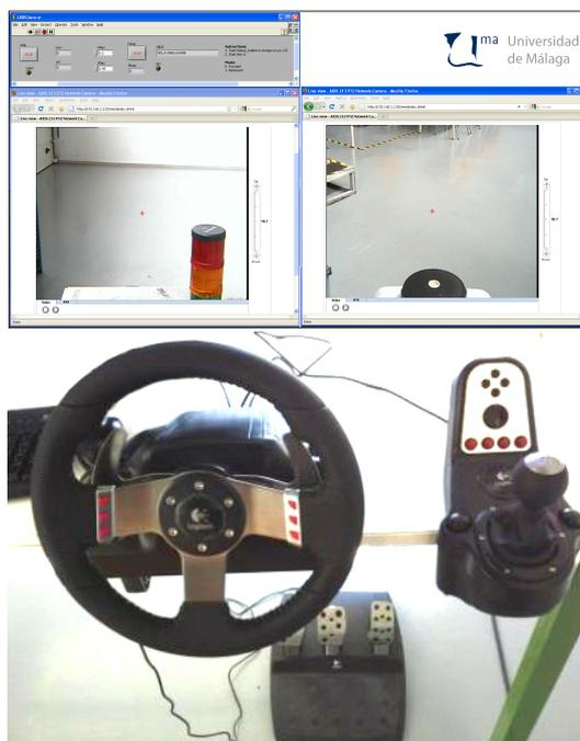
The display offers images from two PTZ cameras for visual feedback: one mounted on the last trailer and another on Auriga- $\alpha$  (see Figure 3). These images are received through a local wireless TCP-IP network, which is independent from the link between the PCs.
