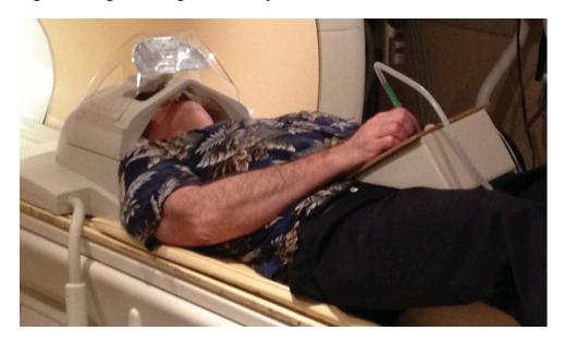
We tested the fMRI-compatible pen with two 11 year-old subjects while they were performing writing tasks in a 3T scanner. Each task was presented in two 4-minute blocks to be used in an fMRI connectivity analysis preceded by a 6 second reminder instruction screen. Stimuli within each block were pseudo-randomly selected.
