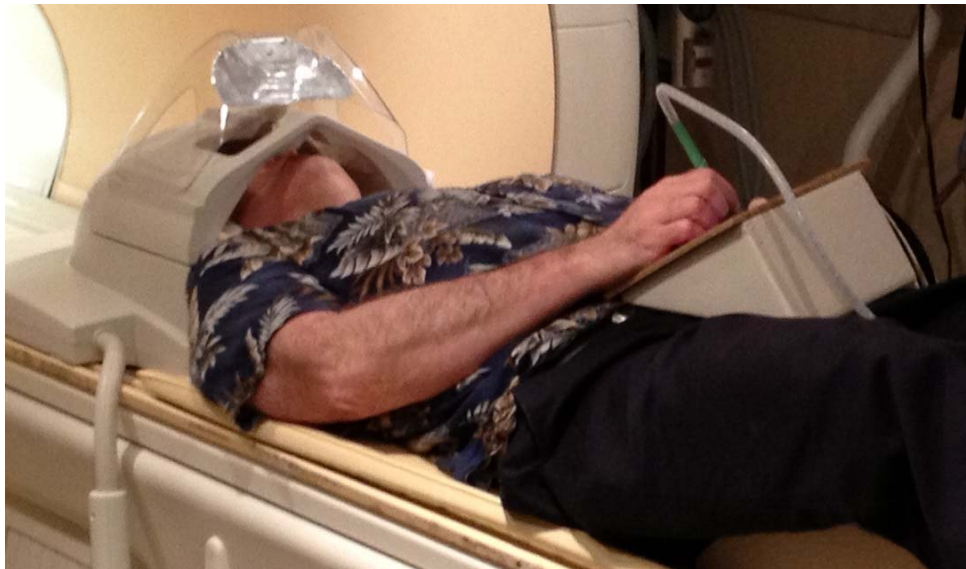
Figure 5. Tablet in use near the bore of the MRI scanner. The pen is connected to a fiber optic cable that goes through a waveguide that is positioned in the wall of the scanner room.
