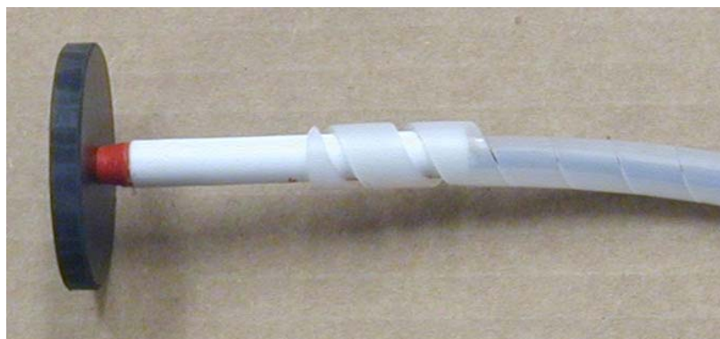
Figure 1. The pen assembly shown prior to securing with glue and enclosure in heat-shrink tubing.
