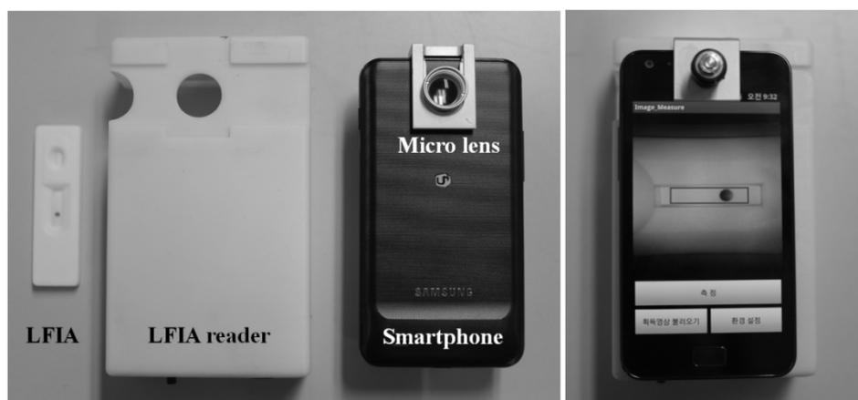
The analysis process of Smartphone-based reading system is as follows. The Smartphone camera was positioned on the close-up lens mounted in the top of LFIA reader. The white LED lights illuminated the detection area of LFIA, and the image of detection area was acquired using the Smartphone camera. The optical density of this image was measured by the Smartphone application,
