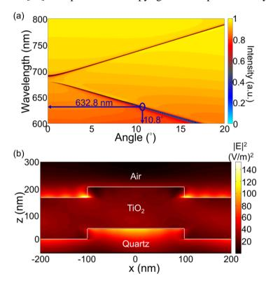
**Figure 3.** (a) Simulated dispersion diagram for the PC used to enhance fluorescence from both Cy-5 and Cy-3 excitation wavelengths. Resonance for the enhanced excitation for the TM mode is  $\theta$ –9.2 °for Cy-5 excitation and  $\theta$ –13.8 °for Cy-3 excitation. Reprinted from [19] with permission. Copyright 2010 American Institute of Physics.
