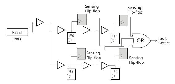
**Figure 11.** Multiple placement of sensing flip-flop.
