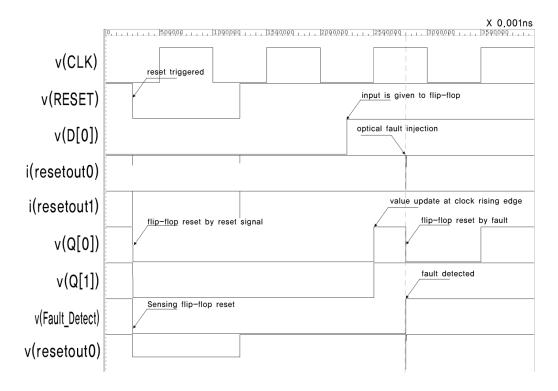
**Figure 6.** Simulation result for the circuit in Figure 3.
