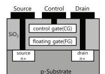
**Figure 1.** Structure of a non-volatile memory cell.
