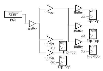
Figure 2. Buffer tree over the reset net.
