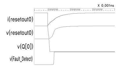
**Figure 7.** Enlarged waveform at the moment when the fault is injected.
