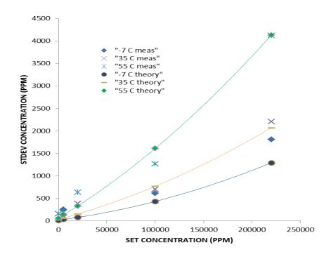
Measured noise is also shown in Figure 15. Dominant noise contribution for temperature <20 °C is Johnston noise and temperature >20 °C dark current noise. Figure 15 shows noise increases with temperature, dominated by dark current noise with increasing temperature.
