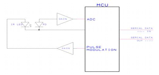
Mid-infrared light level is detected by the PD and is amplified by a GAIN stage before being captured by the MCU's Analogue to Digital Convertor (ADC) thus making a digital version available for processing. The digital version of the IR light level is processed by the MCU which then provides a serial data output indicating the CO<sub>2</sub> concentration present between the mid-infrared LED and the PD.
