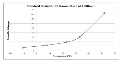
Influence of noise with temperature can be reduced by increased measured signal averaging with time. Data shown in Figures 15 and 16 correspond to standard signal output from wide range and ambient configurations, based on averaged two measurements per second. Noise contributions and variation with temperature for ambient and wide range sensor configurations are similar as same LED/PD combination is used for in both types.
