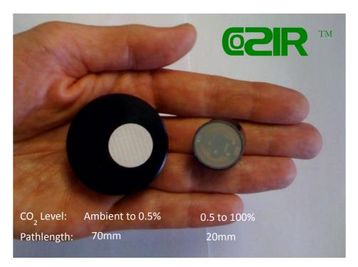
Assembly requires no active alignment of LED/PD bridgeboard and uses low cost plastic optics.
