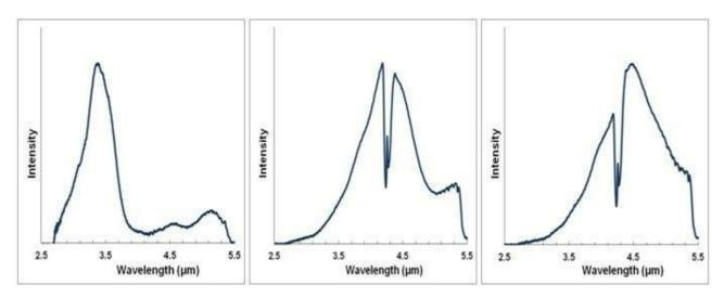
Figure 3(a–c) show measured LED tuned outputs to wavelengths overlapping gas absorption features in the mid infrared—3.3 (methane), 4.3 ( $\rm CO_2$ ) and 4.5  $\mu m$  (carbon monoxide), respectively [the absorption features exhibited in Figure 3(b,c) are due to  $\rm CO_2$  gas within the measurement system]. Figure 4 shows PD spectral response.
