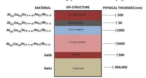
Figure 2. Schematic of narrow bandgap III-V AlGaInAsSb epi-grown structure.
