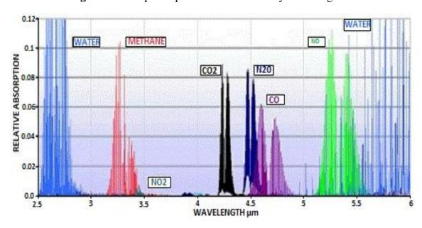
**Figure 1.** Absorption spectra for commercially relevant gases.
