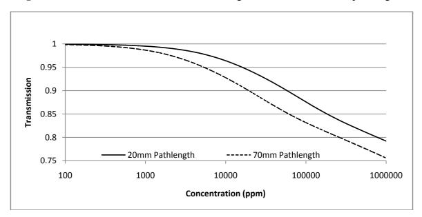
Modelled relative noise (Noise [pathlength 70 mm]/Noise [pathlength 20 mm]) is shown in Figure 8. Figures 7 and 8 show two pathlengths, 20 and 70 mm, are required to provide accurate measurement over ambient to 100% CO<sub>2</sub> gas concentration. 20 mm pathlength is suited to concentration levels from 0.5 to 100% whilst 70 mm pathlength provides complementary required accuracy from 400 ppm to 0.5%.
