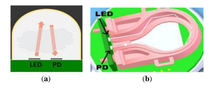
As Shown in Figure 9(a) 20 mm pathlength is a dome geometry with a single reflection, whilst 70 mm pathlength (Figure 9(b)) is achieved with a folded optic and multiple reflections between LED and PD. Both optical configurations are produced using injection moulded optics, reflective surfaces
