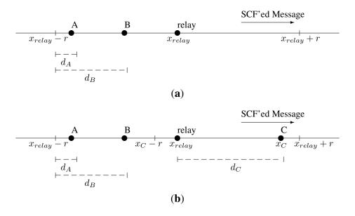
The existence of an unnoticed vehicle in the range,  $(x_{relay}, x_{relay} + r]$ , poses a problem. This case is shown in Figure 8(b). Another vehicle from the range,  $[x_{relay} - r, x_{relay})$ , may be further than r from the new relay. Because it did not hear it, it will forward the message. In addition, it will have to store-carry-forward, because it will not find any other one to become the relay of an old message.
