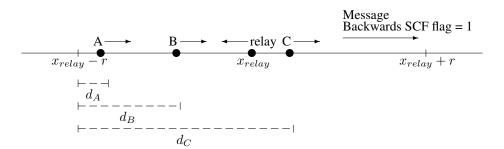
First, they will compute the distance to  $x_{relay} - r$  instead of the distance to  $x_{relay}$ . Then, they will consider a maximum distance of 2r between the closest and the furthest from the origin. The maximum contention time,  $T_{max}$ , must always be the same. All this is reflected in Equation (8):
