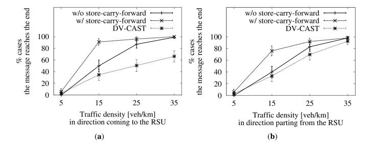
Now, we can see how the success rate, either when using store-carry-forward or not, is better when the traffic density in the direction approaching the RSU is higher. One would think that it should be better when the density in the opposite direction is higher. As these vehicles travel in the same direction as the message, it would have a better chance to get carried by them to the end of the target area. Therefore, this result is unexpected. We will come back to this later.
