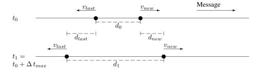
Because of the forwarding scheme, the location of the last relay must be present in the message. In order to make the new relay able to avoid a problematic case, we are going to include the current speed, too. However, to preserve some of the driver's privacy, we do not want to include whether the vehicle is going towards the RSU or away from it. Therefore, the new potential relay will use the most restrictive rule to decide if it is eligible as a relay or not:
