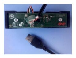
Figure 12. Photo of magnetic card swiping system with USB's interface.
