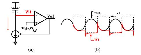
Figure 7. (a) Tracking circuit in the crest tracking state. (b) When  $V_1$  is low, the tracking circuit tries to detect the input crest.
