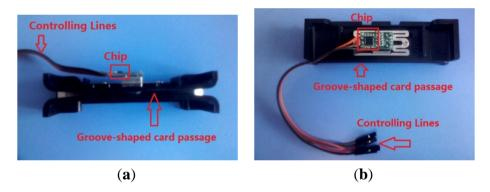
As the figures shown, one side of the chip is connected to the magnetic heads, and the other side is connected to a four-hole slot. The four-hole slot can be used to connect to a micro-processor.
