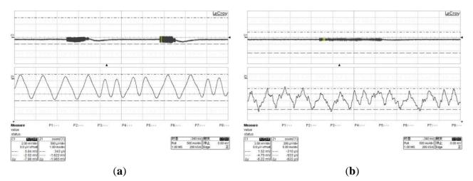
According to the F2F encoding, the sensed signals can be read out as a sequence of binary signals "00000001101000001". When the swipe speed was slow, there were some small spikes in the sensed signals, as Figure 14b shown. However, due to the proposed tracking circuit and AGC with offset correction circuit, the binary signal still could be read out.
