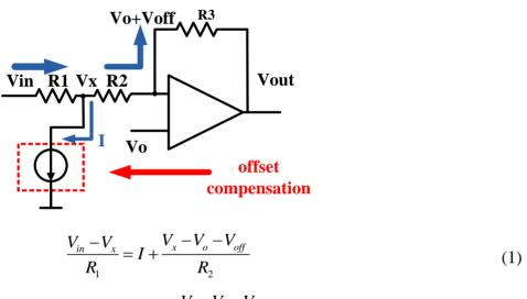
$$V_{o} + V_{off} - V_{out} = R_{3} \frac{V_{x} - V_{o} - V_{off}}{R_{2}}$$
