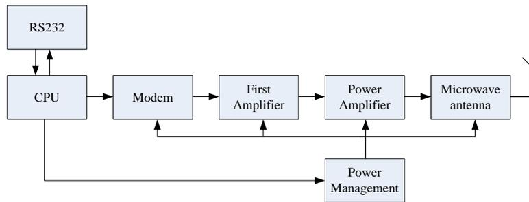
Figure 15. Microwave receiver unit block diagram.
