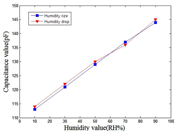
The experimental results showed that the humidity sensor has small humidity hysteresis. As shown in Figure 9, the capacitance of the sensor increased from 100 pF to 150 pF, and the sensitivity of the sensor is about 0.375 pF/%RH. The humidity sensor was tested at 0 °C, +10 °C, +20 °C, +30 °C and +40 °C, in order to characterize the influence of temperature by recording the capacitance changes. The sensitivity of the sensor can be obtained by the linear fitting to the data shown in Figure 10. The
