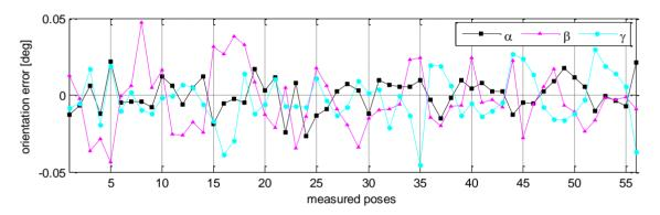
The experimental results for the HA-06 robot show that robot pose accuracy is enhanced significantly after calibration. The proposed measurement method supplied the accurate full-pose measurements for this calibration and had some properties of effectiveness, correctness and practical applicability.
