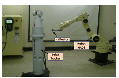
Figure 4. Experimental setup for calibration.
