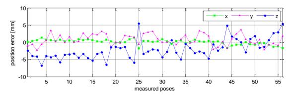
Figure 7. Robot position accuracy after calibration (pose set Q<sub>1</sub>).
