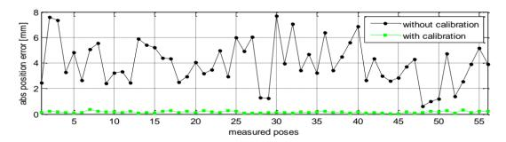
Figure 14. Absolute position accuracy at calibration poses Q<sub>1</sub> and validation poses Q<sub>2</sub>.
