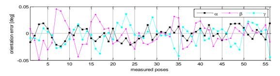
Figure 13. Robot's absolute position accuracy (validation, pose set Q<sub>2</sub>).
