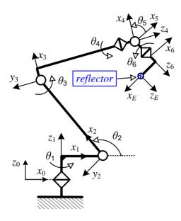
Figure 5. Schematic of robot HA-06 and attached link frames.
