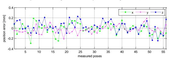
Figure 11. Robot position accuracy (validation, pose set Q<sub>2</sub>).
