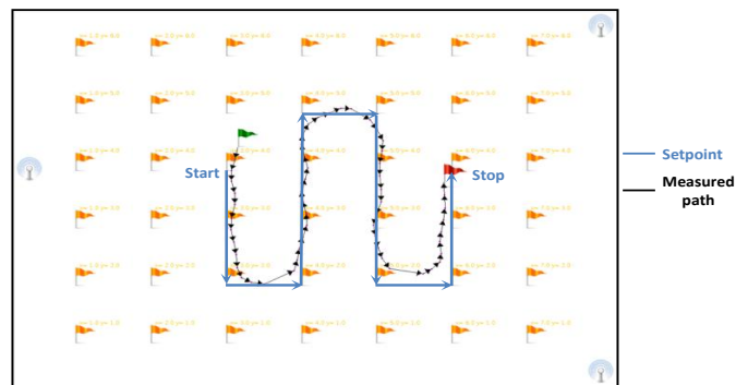
Figure 13. Path filtered by the post-processing software.
