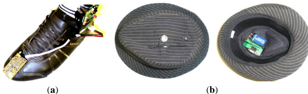
Figure 7. (a) Device embedded on a shoe. (b) Device embedded in a hat.
