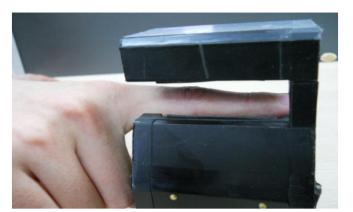
Figure 6. The finger vein image capture device.
