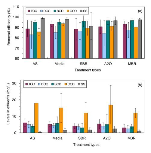
The TOC, DOC, BOD, COD and SS removal efficiencies were not statistically distinguished among the five different treatment types (ANOVA, p > 0.05), except for the lower removal efficiency of COD using the AS treatment than using the Media treatment (86% ± 3% vs. 94% ± 2%, Table 1; ANOVA, p = 0.04). The levels of TOC, DOC, BOD, COD and SS in the effluents showed no significant difference among the five different treatment types (ANOVA, p > 0.05; Figure 1b).
