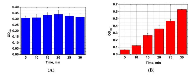
Next, ELISA assays with varying Step A duration from 5 to 30 min were compared. As the results in Figure 3 show, the signal intensities (levels achieved in the absence of the competitor) differed by less than 10% across the time intervals tested. Thus, even 5 min incubation was sufficient for near complete immune interaction. Additional reduction of Step A was impractical because a higher degree of error
