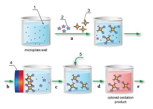
Step a: Free AFB1 contained in the test sample competes with peroxidase-labeled AFB1 for binding sites on the antibodies adsorbed on the MNP surface.
