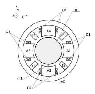
As shown in Figure 5, the displacement sensor probe (T1~T4) is mainly composed of a crystal oscillator, AGC network, resonant circuit, filter circuit and amplifier output circuit. The crystal oscillator is used to provide a stable frequency and amplitude for the excitation signal.
