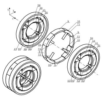
A-magnetic bearing, D-coil, T-sensor probe, 9-permanent magnet, 10-sensor base.
