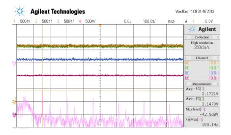
**Figure 17.** The current curves of every channel when the temperature of the sensor probe is at 98  $^{\circ}$ C.
