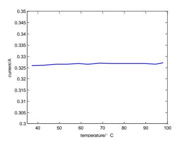
Figure 15. The relationship between temperature and coil current.
