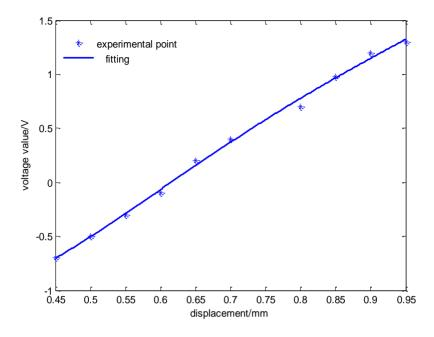
Figure 13. The relationship between displacement and output voltage value.
