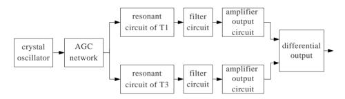
As we know, the principle of the eddy current displacement sensor is the mutual inductance effect between a high frequency current in coils and detector. Therefore, the detector material has an important influence on the sensitivity and precision of the displacement sensor. Steels such as 45# or 40Cr can often be used considering their stability.
