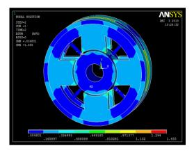
Figure 10. Flux density distribution of the stator in the proposed structure.
