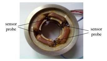
Figure 12. Photograph of a HSMSM with the proposed structure.
