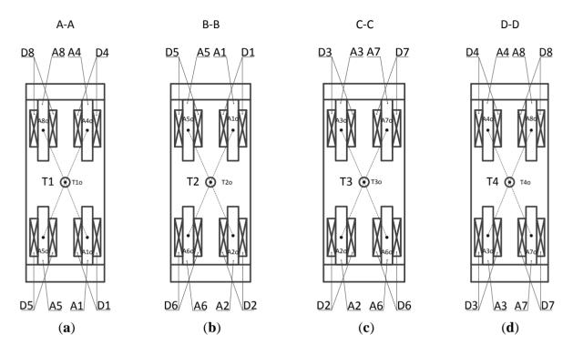
In practical fact, a pair of differential output probes is composed by sensor probes (T1, T3) as well as the other sensor probes (T2, T4). As shown in Figure 4, an air gap is formed between magnetic poles (A1~A8) and rotor (R) and the detection gap is formed between sensor probes (T1~T4) and rotor (R). The length of the air gap (m1, m2) is designed to be 0.4~0.5 mm and the detection gap is designed to be 0.75~1.25 mm.
