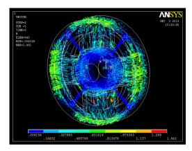
Figure 8. Flux distribution of the proposed structure.
