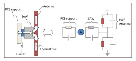
Figure 8. QUCS model of the WiPirani prototype.
