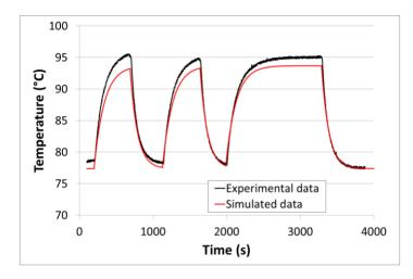
As will be shown in Section 3, the huge response time was due to the big size of the prototype's building blocks, especially the bulky antenna used for the interrogation of the SAW sensor. The big size of these components implies a big thermal inertia and therefore a long response time. Ways to strongly improve the response time will be discussed in Section 3. We believe that the response time can be made smaller than a few seconds, especially if MEMS technology is employed.
