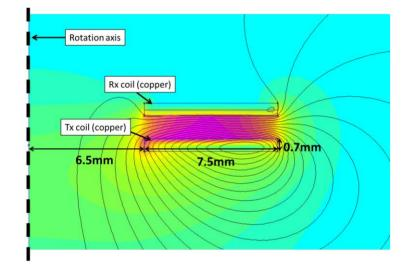
Figure 5. FEMM Model of the power transmission component of the WiPirani.
