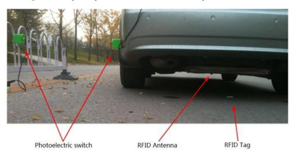
Figure 7. Setup of experimental verification based on photoelectric switch.
