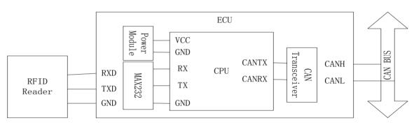
Figure 3. The connection of RFID reader and ECU.
