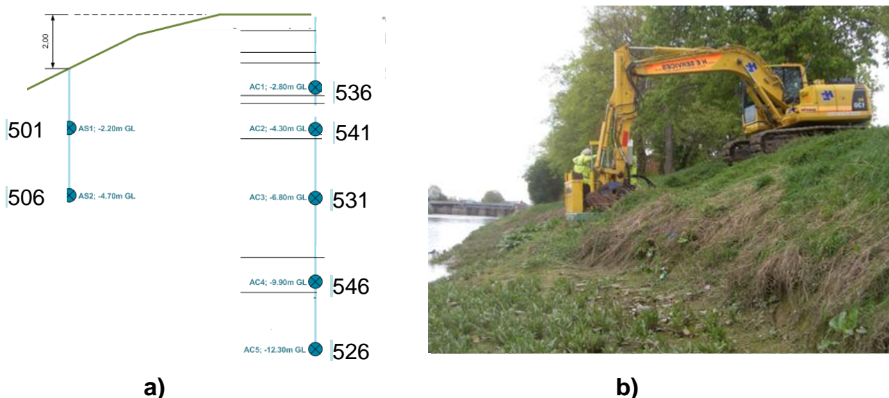
Figure 20. (a) One of two cross-section of the Boston levee, circles with numbers show installed pore pressure sensors. (b) A photo of the Boston levee.
