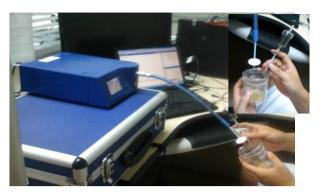
Figure 3. Sampling set-up using the electronic nose.
