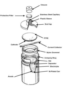
Figure 1. Early version of lead-based electrochemical sensor (modified from [8]).
