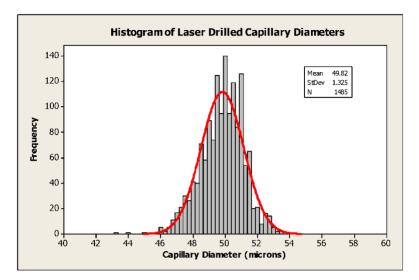
Figure 4. Sensor capillary diameters—typical reproducibility of development samples.
