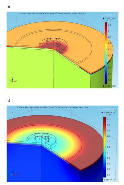
**Figure 8.** Example of electrochemical oxygen pump model outputs. Lifetime predictions for continuous operation at selected temperatures and relative humidities.
