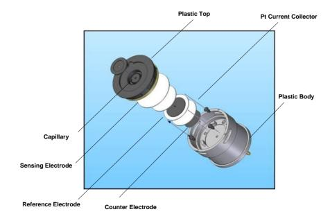
Figure 5. Early design for liquid electrolyte fuel-cell oxygen pump.
