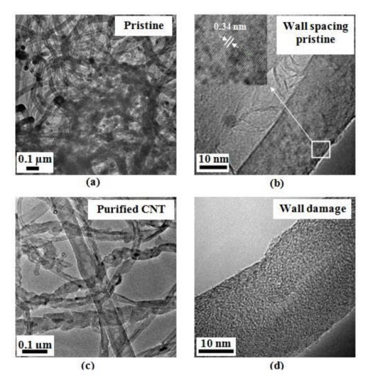
TEM images of Pd decorated CNTs are shown in Figure 3. Heterogeneous nanotubular morphology with the tubular structure is partially destroyed by the aggressive acid treatment is shown in Figure 3a. Pd NPs were found on the outside walls and the tips of MWCNTs. No agglomeration is observed after the decoration process. Defects serve as anchor by attachment of functional groups and NPs. The
