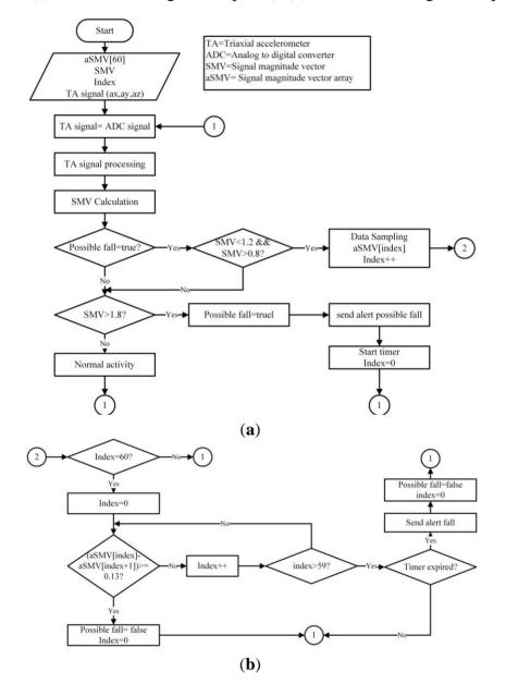
Figure 3. (a) Fall detection algorithm (part 1); (b) Fall detection algorithm (part 2).
