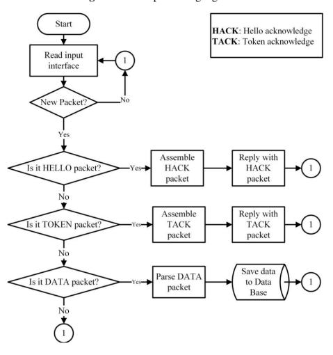
**Figure 5.** SINK processing algorithm.
