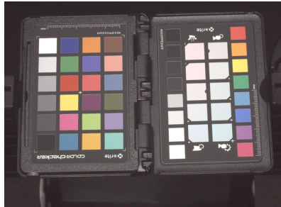
Figure 13. The X-Rite ColorChecker Passport. The color chart is used to calibrate the cameras' color profiles in the Dome 1 and Dome 2 as well as the cameras' response functions of the Dome 2.
