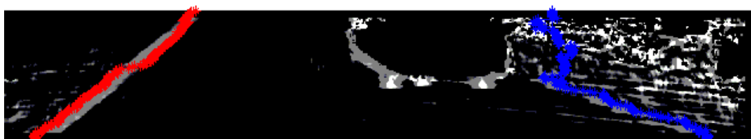
Figure 14. Best path for each side. Red points indicate the left curb, blue points indicate the right curb.
