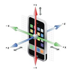
The mobile device is located on the central part of the waist, corresponding to the body's center of gravity. For maintaining the acceleration axis, the device is fixed in a special phone case attached to the user's belt. The process is split into three main stages. The system starts to receive data from the accelerometer and calculates the overall acceleration value Act:
