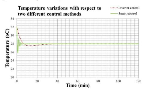
Figure 20. The temperature responses of smart control and Inverter control.
