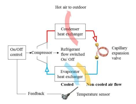
Under the On-Off control structure, the fixed frequency air conditioner turns on the compressor when the return air temperature is higher than the set one, and turns it off on the contrary. By doing this, the refrigerant would flow through the condenser and evaporator for heat exchanging with the indoor and outdoor air to keep the indoor temperature stable. The control scheme is described in Figure 7.
