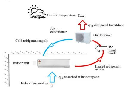
**Figure 2.** Working principals of a split type air conditioner. Smart control design will be applied to this type of air conditioner.
