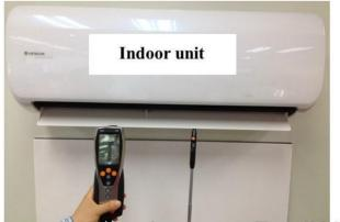
Temperature sensor and anemometer (Testo 435-2) for measuring the indoor temperature and wind speed
