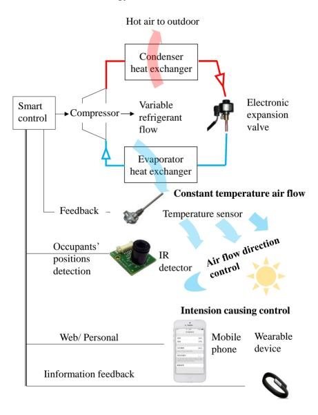
In this paper, the smart control logic will be developed from the air conditioning principles and the controlling logics of fixed and convertible frequency air conditioners. Figure 12 presents the developed smart control scheme developed using the Matlab software. The control scheme is based on the mathematic analysis of Section 2. It will be carried out in the electric circuit after the stability analysis of the control method.
