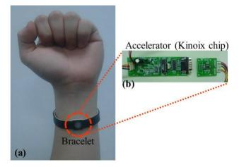
Figure 10. Smart sensor 2: (a) bracelet combining with (b) accelerator (Kinoix chip).
