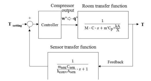
It is noted that, in Figure 5, a closed-loop air conditioning space model includes the room transfer function and sensor transfer function. The thermal mass of temperature sensor, located in the center of evaporator, would cause the convection effect of air flow and the temperature difference between the return air and sensor. The detail of the sensor transfer function is further shown in Figure 6.
