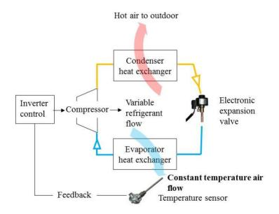
Comparing with the fixed frequency control, the convertible frequency type could first rectify the 60 Hz electricity into the direct current type, and then modulate the frequency of output electricity continuously by pulse width modulation (PWM). According to the feedback temperature difference, the air conditioner could provide the air flow of stable temperature to control the temperature of indoor space by adjusting the refrigerator flow.
