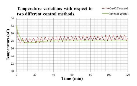
Figure 17. The indoor temperature responses of the Inverter and On-Off controls.
