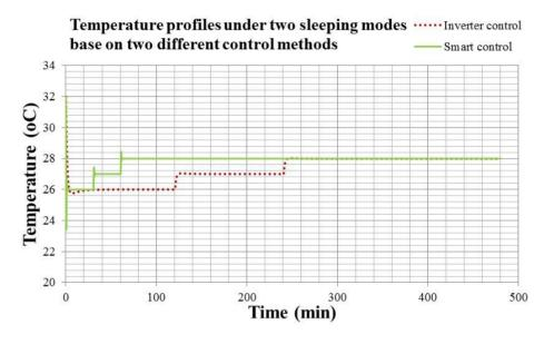
**Figure 22.** The compressor output of sleeping functions in the night under the Inverter and smart controls.
