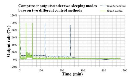
In Figures 21 and 22, the dotted line is the information of Inverter control, and the solid line is that of the smart control. Comparing the results in Figures 21 and 22, it is noted that the smart air conditioner with wearable devices could detect the human temperature and action during sleep for determining the
