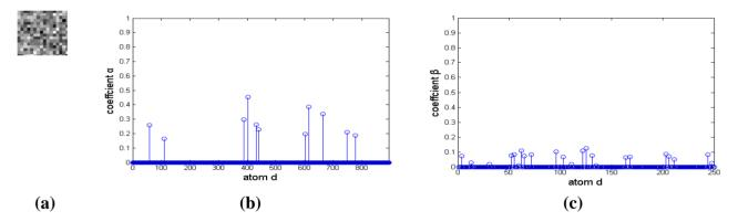
Figure 15. Representation coefficient of background block decomposed in cloud image on discriminative over-complete dictionary. (a) Sparse coefficient on background dictionary, (b) Sparse coefficient on target dictionary.
