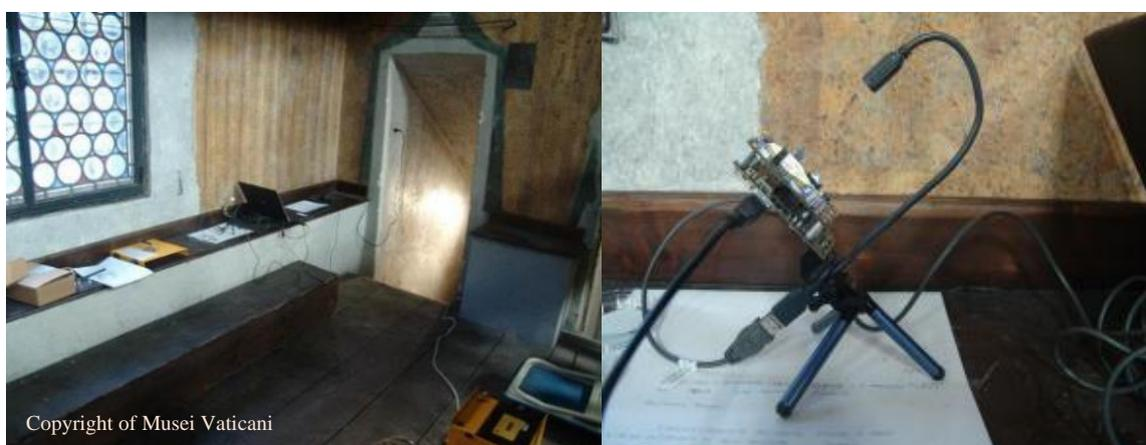
The sensor was placed with a 45° tilt angle (Figure 7). In this way, the dust will be unable to accumulate permanently (as might occur with a horizontal surface) and unable to immediately fall from the sensor (as might occur with a vertical surface). The acquisition time interval was 30 min, in order to have a high number of images to analyse. The acquisition session took two weeks, at the end of which the sensors provided about 750 images. Before its positioning, the sensor has been cleaned
