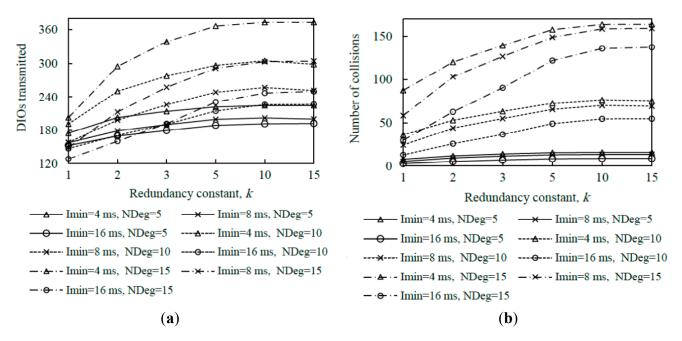
Figure 13. Average number of DIO messages transmitted and collisions in the large network scenario for different average node degrees, as a function of the redundancy constant, k, for different values of  $I_{min}$ .
