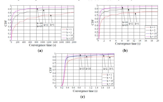
**Figure 8.** CDF of nodes join time for an average node degree of 5: (**a**) small, (**b**) medium, and (**c**) large network size scenarios.
