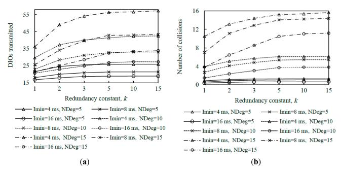
Figure 12. Average number of DIO messages transmitted and collisions in the medium network scenario for different average node degrees, as a function of the redundancy constant, k, for different values of  $I_{min}$ .
