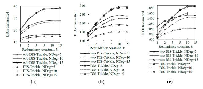
Figure 18. Influence of using DIS-Trickle on the number of DIS messages transmitted in the small, medium and large networks, for different average node degrees as a function of the redundancy constant, k. when the  $I_{min}$  value is set to 8 ms. (a) Small network size, (b) medium network size, and (c) large network size.
