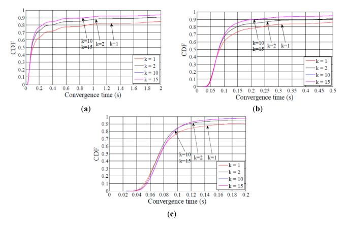
**Figure 6.** CDF of network convergence time in the medium network size scenario. The average node degrees are 5, 10 and 15 in figures (**a**), (**b**) and (**c**), respectively.
