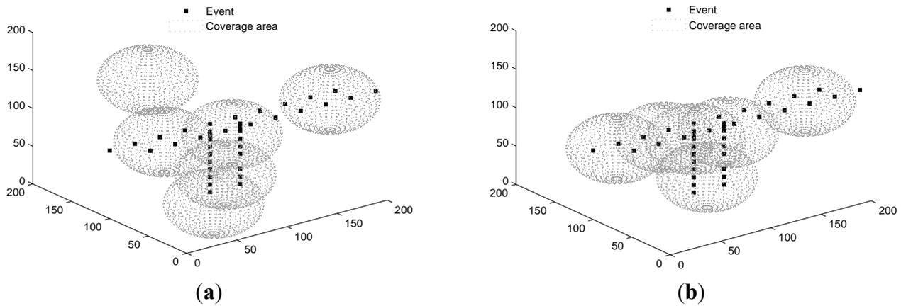
**Figure 6.** Events distributed non-uniformly along a line. (a) solution of SOM; (b) solution of PSSD.
