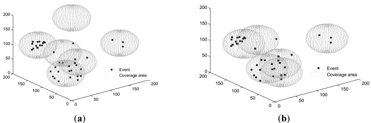
**Figure 5.** Events distributed non-uniformly in T-shape. (a) solution of SOM; (b) solution of PSSD.
