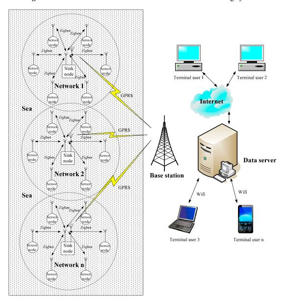
Figure 1. Common architecture of WSN-based marine monitoring systems.
