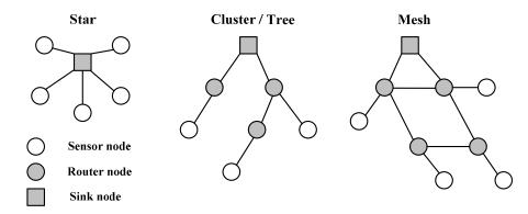
(1) *Star topology:* A star topology is a point-to-point single-hop architecture in which each sensor node connects directly to a sink node. It potentially uses the least amount of power among the three topology architectures.
