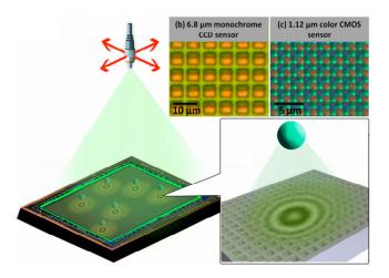
Navruz and colleagues proposed an opto-mechanical add-on which can be attached to the camera of the cellphone, as illustrated by Figure 18 [87]. The purpose of this study was to realize a portable and compact cellphone-based contact microscopy platform, or contact scope, which could image highly dense or connected samples in transmission mode with a relatively higher spatial resolution. Inside this
