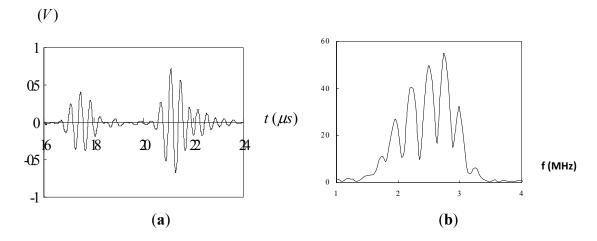
**Figure 10.** Reflection from a surface crack with 1 mm crack depth using 5 MHz longitudinal wave: (a) time domain; (b) frequency domain.
