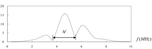
**Figure 8.** Fourier transform of two pulses with time delay  $\Delta t = 0.55 \mu s$ .
