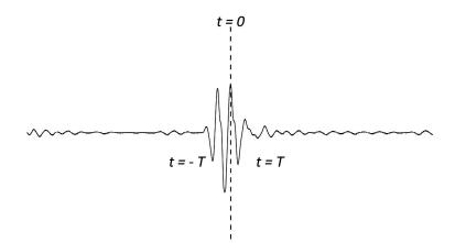
Figure 4. Two identical ultrasonic pulses with time delay of  $2 t_0$ .
