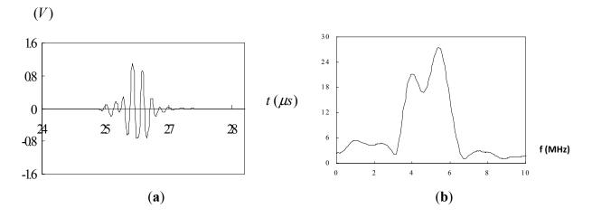
Figure 11. Reflection from a surface crack with 4 mm crack depth using 10 MHz longitudinal wave: (a) time domain; (b) frequency domain.
