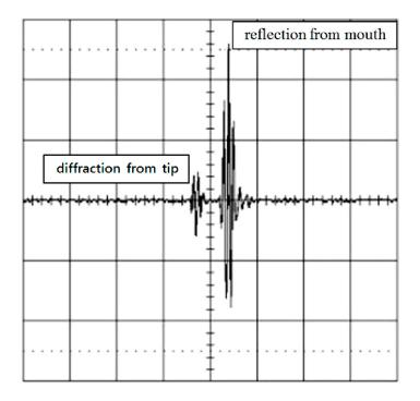
The difference of the travelling paths between the wave diffracted at the tip and the wave reflected from the crack mouth shown in Figure 1 can be calculated as
