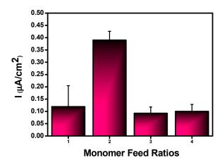
**Figure 5.** Effect of monomer feed ratio on the biosensor response (SNS-NH<sub>2</sub>/SNS-NH<sub>2</sub>-Fc ratios: (1): 0.5/4.5 mg; (2): 1.0/4.0 mg; (3): 2.0/3.0 mg and (4): 5.0/5.0 mg: in sodium acetate buffer, 50 mM, pH 4.5, +0.45 V, [Glucose]: 5.0 mM). Error bars show standard deviation.
