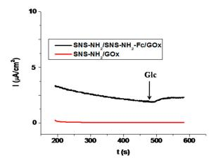
**Figure 7.** A typical chronoamperometric signal of SNS-NH<sub>2</sub>/SNS-NH<sub>2</sub>-Fc/GOx and SNS-NH<sub>2</sub>-Fc/GOx biosensor after glucose addition (in sodium acetate buffer, 50 mM, pH 4.5, +0.45 V, [Glucose]: 5.0 mM).
