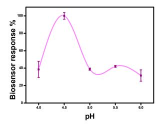
**Figure 4.** Effect of pH (in sodium acetate buffer, 50 mM, at pH 4.0–5.5 and in sodium phosphate buffer at pH 6.0; SNS-NH<sub>2</sub>/SNS-NH<sub>2</sub>-Fc: 0.5/4.5 mg; +0.45 V, [Glucose]: 5.0 mM). Error bars show standard deviation.
