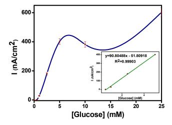
**Figure 6.** Calibration curve of SNS-NH<sub>2</sub>/SNS-NH<sub>2</sub>-Fc/GOx enzyme electrode (in sodium acetate buffer, 50 mM, pH 4.5, +0.45 V).
