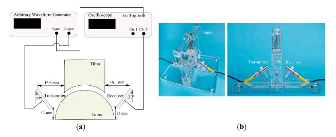
**Figure 4.** (a) Schematic presentation of the experimental setup; (b) Perspex frame designed to hold the tibia and the talus parts. Holders for transducers are included to fixate them at the desired positions.
