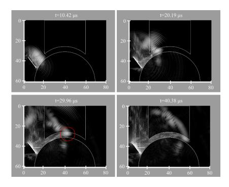
**Figure 10.** Simulated ultrasound pulse at  $t = 10.42 \ \mu s$ , 20.19  $\mu s$ , 29.96  $\mu s$  and 40.38  $\mu s$ . The white bar is the transducer acting as transmitter. Red circle is used to emphasize US pulse guided along the tibia rim.
